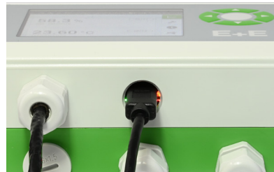
Fig. 28 Plugged USB cable and LED indication
