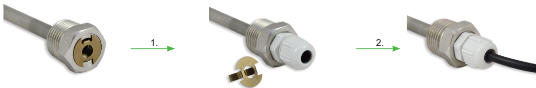
Fig. 15 Handling of the immersion well
