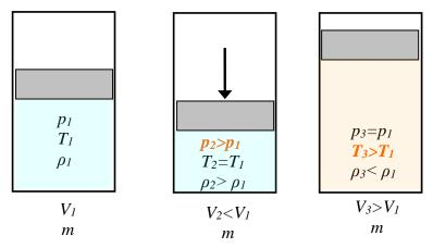
The system is absolutely leak proof, amount and mass of the filled medium is constant. To increase the pressure inside the cylinder the piston is pressed downwards ( $p_2 > p_1$ ), the gas is compressed, the density of the gas is increasing, the volume is decreasing. On the other hand, by heating the gas inside the cylinder ( $T_3 > T_1$ ), the density of the gas is decreasing and the volume is increasing!
