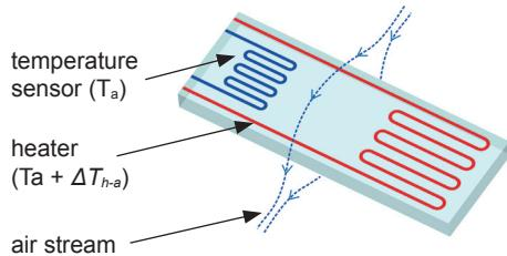
An E+E air velocity sensor consists of two resistors deposited on a thin glass substrate. One resistor is used as temperature ( $T_a$ ) sensor and measures the temperature of the ambient air flowing along the sensor ( $T_a$ ).
